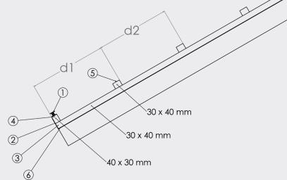
Air is allowed to flow in through the lowest part of the roof at the eaves by keeping the space between the roof support and the tiles open. Eaves grates and/or combs cover the space under the eaves, preventing birds from entering the gap while allowing air to circulate. The combination of FLAT-5XL ceramic tiles and SOLAR FLAT-5XL ceramic roof tiles means that the perimeter of the roof must always be completed using FLAT-5XL ceramic tiles and their complementary accessories.
