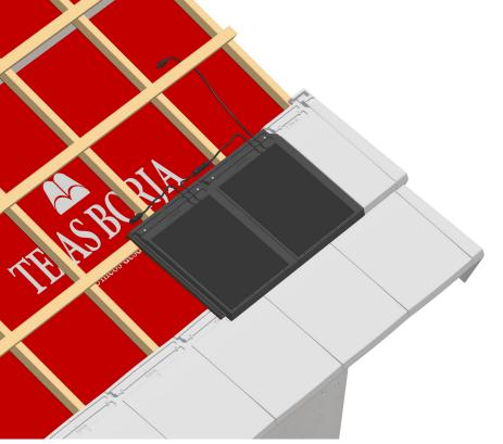
Position the second **SOLAR FLAT-5XL ceramic roof tile** so it overlaps the previous solar tile which has just been installed. Fix the second tile in place using 2 screws, making sure the connection cables and connectors are always kept in view and beneath the secondary batten.
