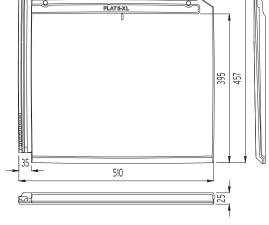
$\label{eq:continuous} \textbf{Approximate values:} \ \ \text{If the roof tiles are installed on battens, the useful length must be calculated on site.} \ \ \text{A tolerance of $\pm 2\%$ is allowed on the dimensions of the roof tiles according to EN 1024.}$
