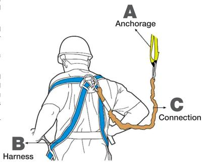
Fall protection system for working at height
