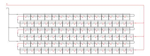
Wiring diagram for the system with SOLAR FLAT-5XL ceramic roof tiles
