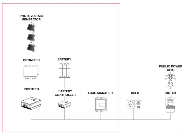
The maximum number of solar tiles which may be connected in series depends on the system design, the type of inverter used and the environmental conditions.
