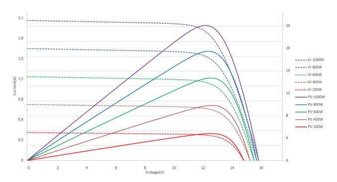
I-V and P-V curves - SOLAR FLAT-5XL ceramic roof tile MONOCRYSTALLINE
