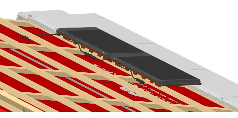
NOTE: When making any connection using MC4 connectors, you will hear a click if you make the connection correctly. Locate the cables behind the solar tile and fix them to the secondary batten using corrosion-resistant clamps in such a way that the connections will never come into contact with the roof supports.
