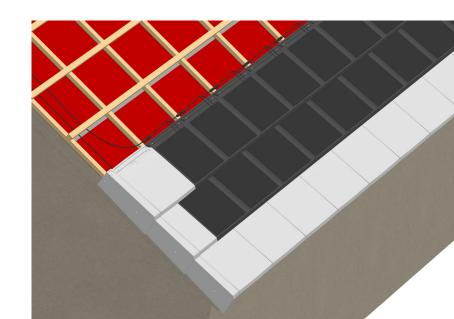
Complete the array with all its component strings, installing a FLAT-5XL half tile in alternate rows. Follow the same installation steps and complete the fixings and connections following steps 1, 2, 3, 4, 5, 6, 7, 8 and 9, finishing on the left side of the roof with a FLAT-5XL tile and edge piece (step 6), installing a FLAT-5XL half tile in alternate rows (step 9).
